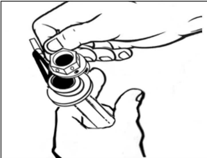
**Fig.2 Placing the Adaptor on the Ice Screw**
