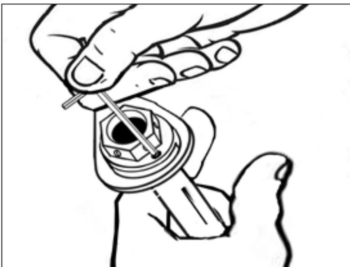
**Fig. 3 Tighten set screw** on Adaptor with the Hex Wrench (supplied) so the Adaptor does not come off the ice screw. Thread lock on set screw will help keep screw in place. **Caution** – Do not loosen set screw after tightening. If you do, you must add thread lock again to help keep set screw in place during use.
